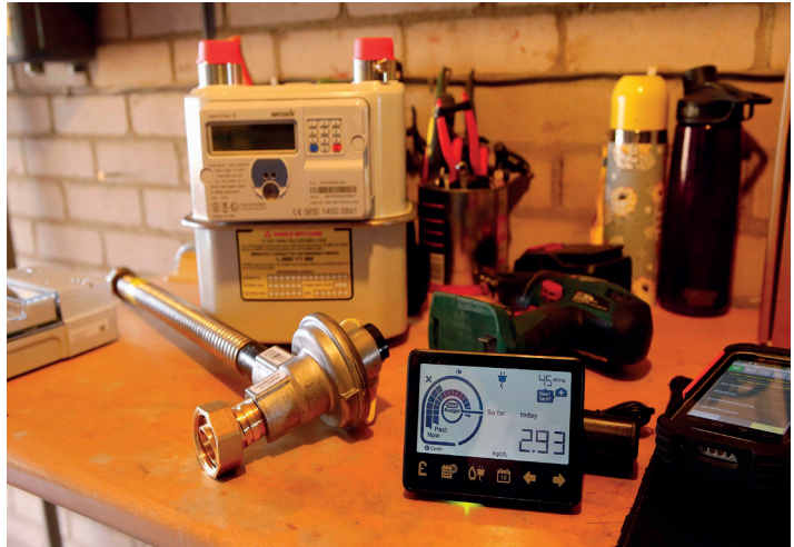
A smart meter and an In-Home Display
